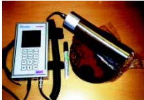
*A measurement of a piece of the pressure hull from compartment VIII is performed by use of the EasySpec multichannel analyser with the NaI detector.*
