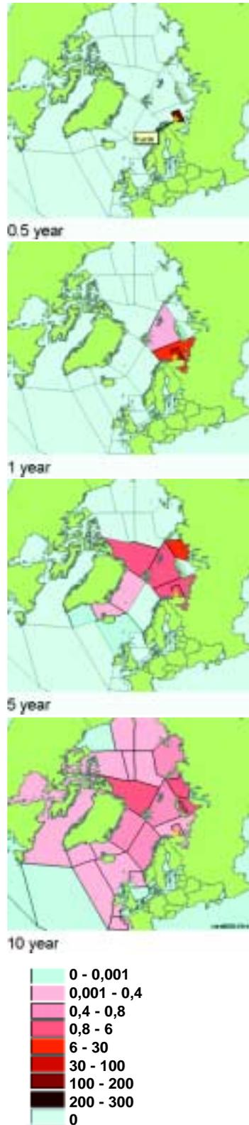
Fig. 12) Dispersion of  $^{137}\text{Cs}$  ( $\text{Bq m}^3$ ) after a potential release of radionuclides from the submarine the Kursk into the Barents Sea.
