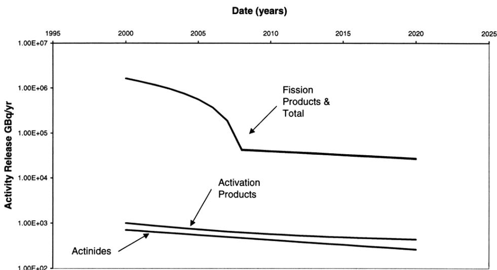
Fig.11) Activity released from reactor pressure vessels in a sunken submarine (NATO Pilot Study, 1999).
