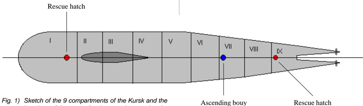
Fig. 1) Sketch of the 9 compartments of the Kursk and the locations of the ascending buoy and rescue hatches.
