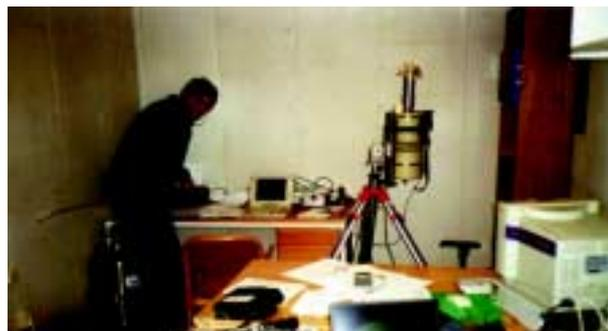
The mobile laboratory at the Regalia. A HPGe detector, mounted on a stand is shown in the back.
