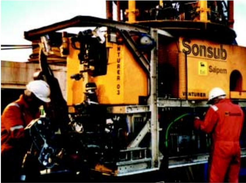
Two operators are preparing the ROV for a new working period.
