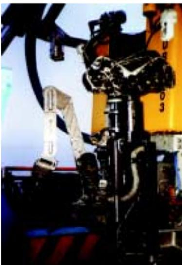
Front part of the ROV is shown with the titanium arm (left) and the dose rate meter in the water-proof housing (upper left).
