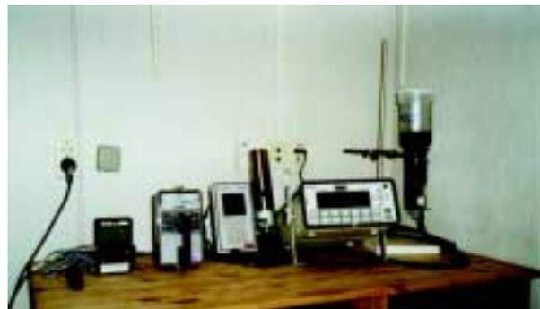
Some of the equipment at the mobile laboratory on the Regalia. From left: Automess dose rate meter; Bicron dose rate meter; EasySpec with 2" x 2" NaI detector; Canberra serie 10+ with 3" x 3" NaI detector with a 200 ml. sample box on top.
