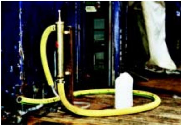
*Water sampling device used for collecting water from inside the submarine at the Regalia expedition. Flexible rubber tubes (yellow) were lowered into Kursk and into a 25 litres plastic container.*
