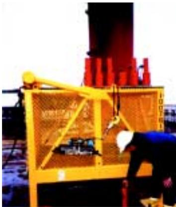
A rack of six corers, used for sediment sampling (red colour), is mounted on top of the basket. The Nansen water sampling device is mounted in front of the basket.
