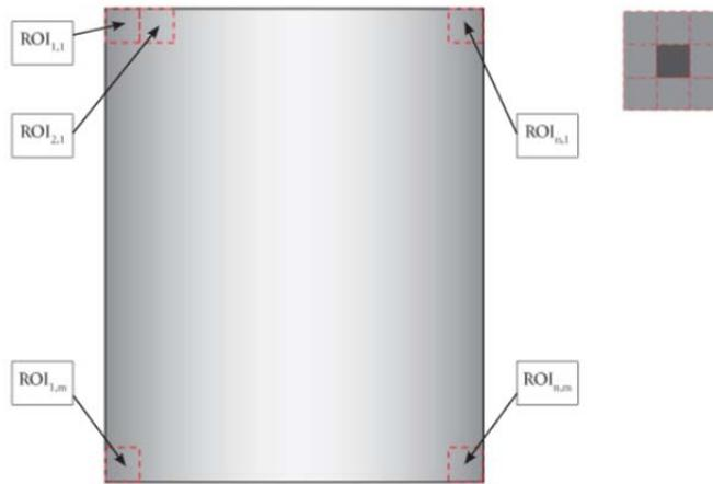
**Figure 3** Illustration of naming convention for ROIs. The image is divided into a matrix of quadratic elements  $ROI_{i,j}$ , each with a middle pixel value  $MPV_{i,j}$ . A single ROI together with its eight neighbouring ROIs are represented on the upper right side of the image.
