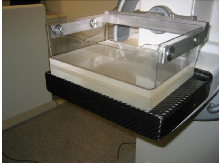
**Figure 1** Image acquisition set-up: Perspex phantom covering the detector is subjected to x-ray exposures.
