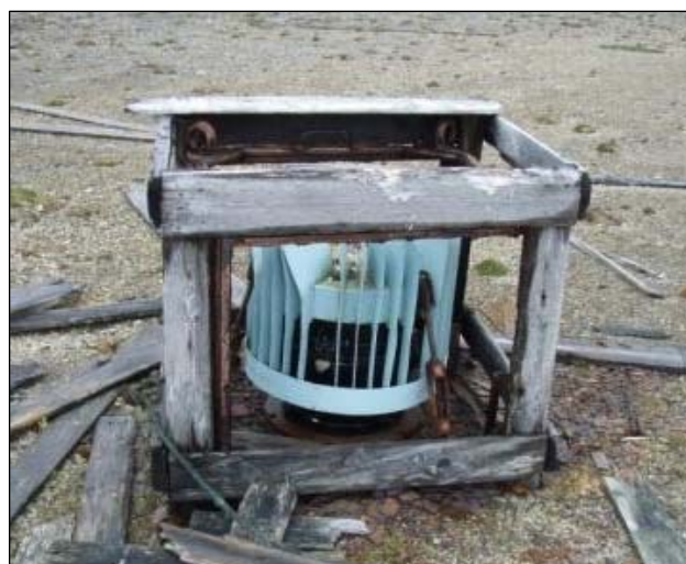
A defective RTG. Photo: County Governor of Finnmark.
