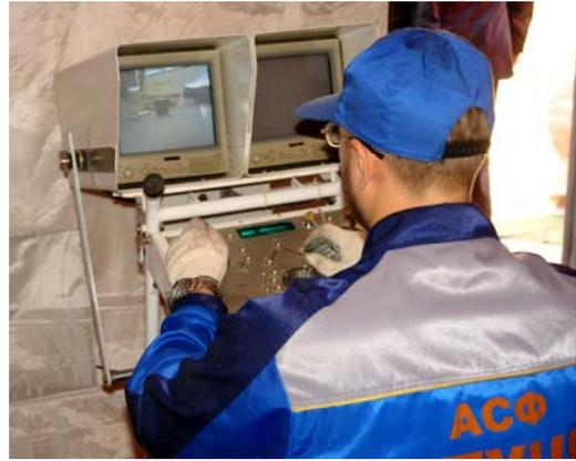
*Mobile remote control system taking control over radiation heat source RHS -90. Photo: NRPA.*
