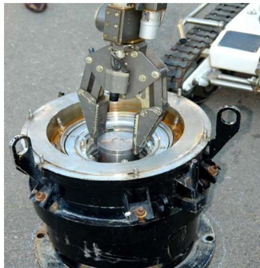
*Regaining control over RHS-90 source, its placement in a shielded container for forward disposal. Photo: NRPA.*
