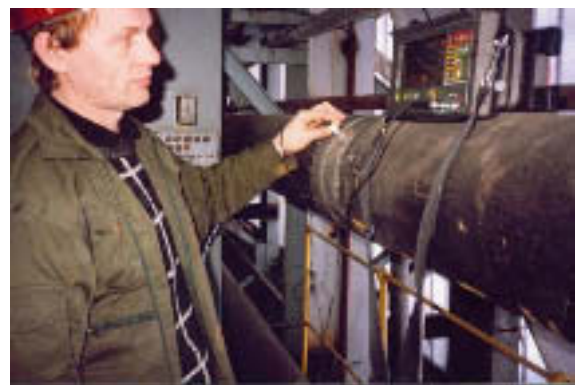
Figure 3-5: Ultrasonic inspection (Photo: IFE)
