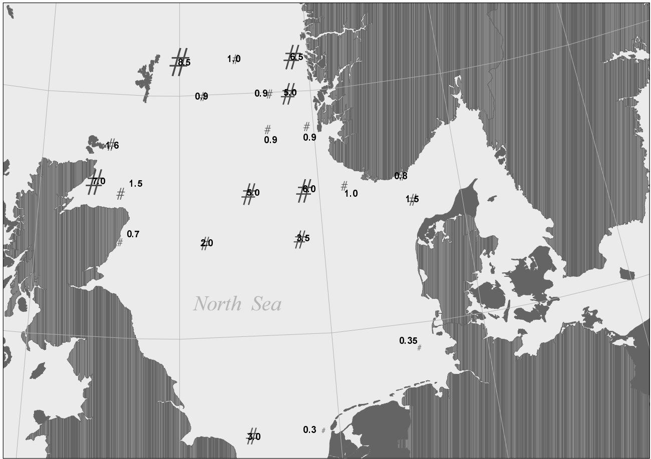
Figure 2 : Levels of 99 Tc in seawater for the North Sea and Norwegian coastal waters in November 1996.
